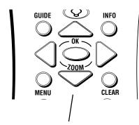
These are the buttons on the remote you use to navigate through the monitor's on-screen menu system.
